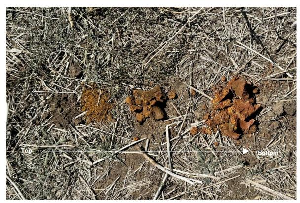
Photo 3: Excavated material from borehole 1.
